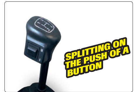
The 8 forward gears are subdivided into 16 gears by the splitting ("half gear") group, creating an even finer speed stepping.
