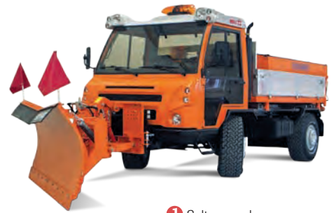
1 Salt spreader 2 Snow plough
