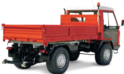
1 3-side tipper 4 Rear linkage
